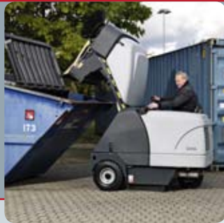
The Nilfisk SR 1601 features a "high-dump" hopper emptying system, capable of dumping into standard containers
